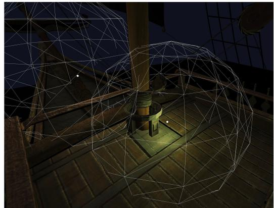
**Figure 1:** Two light volumes visualized as polygonal spheres in the render engine used for this project, using an attenuation threshold of 0.3. In practice, a smaller attenuation threshold would be more typical for light culling; for evaluation, this paper uses a threshold of 0.02. Image contrast is increased for clarity.
